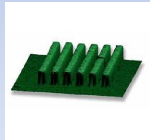
SPM image of 70 nm photoresist lines.
